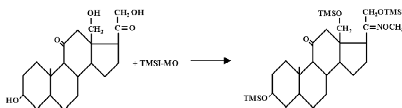
Fig. 2. TMSI-MO derivatisation of 18-OH-THA. Three (OH) groups at C-3, 18, 21 were silylated and the keto group at C-20 was methoximated.
